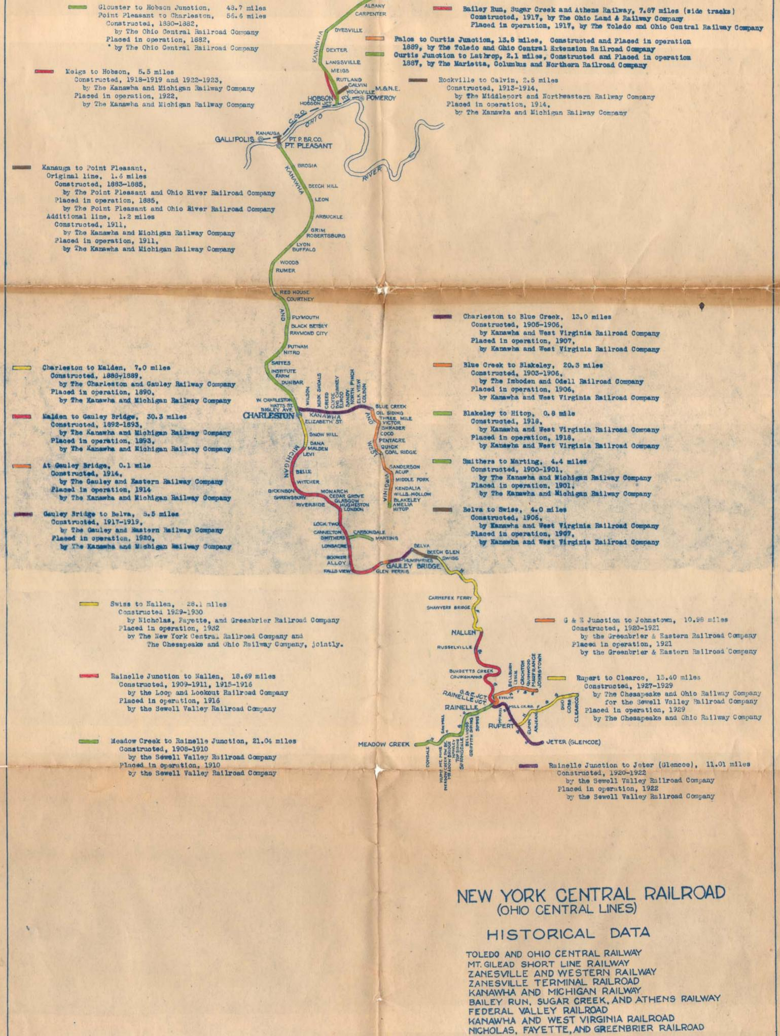
Note .- There are some minor discrepancies between mileage figures hereon and original construction mileage. Adjustments have been made so that mileage figures appearing on this map are applicable to present road.
