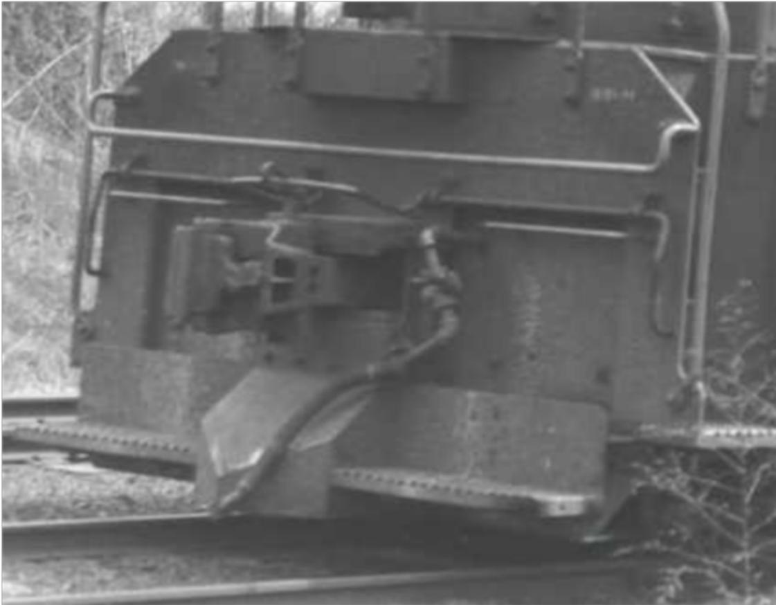
*A close up view of unit 8588's front end shows the addition of tubing used to supply water to the rail washer. In the lower right a portion of the rail washer can be seen.*
