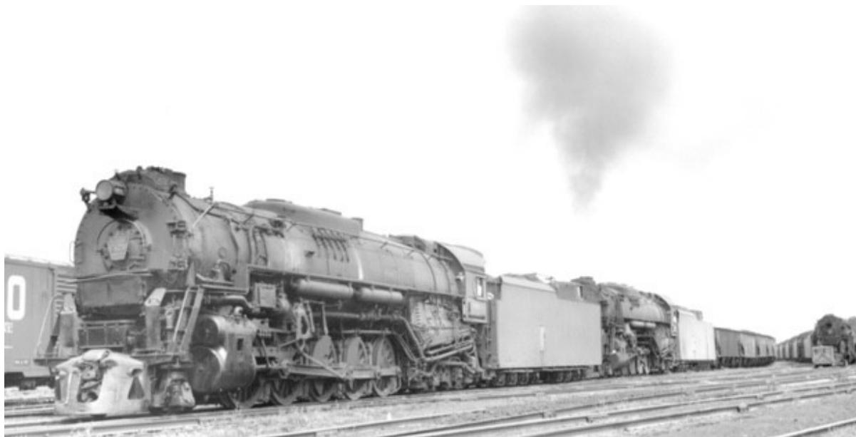
*Pennsylvania Railroad Class J1 2-10-4 No. 6478 in the lead, passing the Chase Avenue Yard with a coal drag heading to Logansport on the Bradford Line. Photo from Ryan Hoover Collection.*
