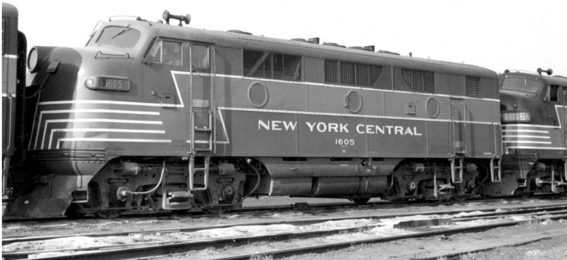
**F2 No. 1605 taken at the West Columbus Yard. Photo by Galen Gonser, April 1958. Note the small stirrup and grab iron just forward of the front truck wheels. The model F “covered wagons” were built for over-the-road haulage and viewer esthetics, but not for the brakeman’s comfort and safety while switching.**
